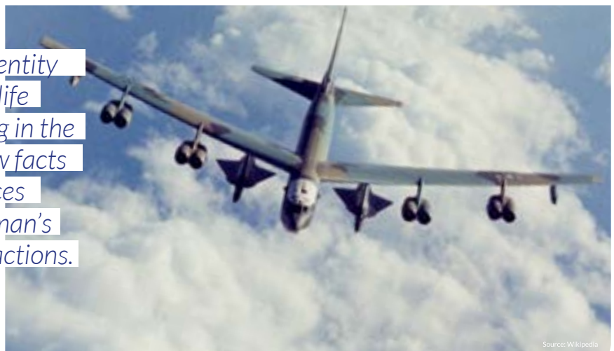
B-52 acted as mothership, carrying under its wings two Lockheed D-21 (surveillance Unmanned Aerial Vehicle)
